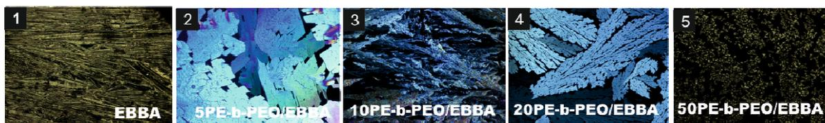
**Figure 1.** OM micrographs of a1) HOBC and PE-b-PEO/HOBC blends with 2) 5, 3) 10, 4) 20 and 5) 50 wt % of PE-b-PEO block copolymer and b1) EBBA and PE-b-PEO/EBBA blends with 2) 5, 3) 10, 4) 20 and 5) 50 wt % of PE-b-PEO block copolymer.
